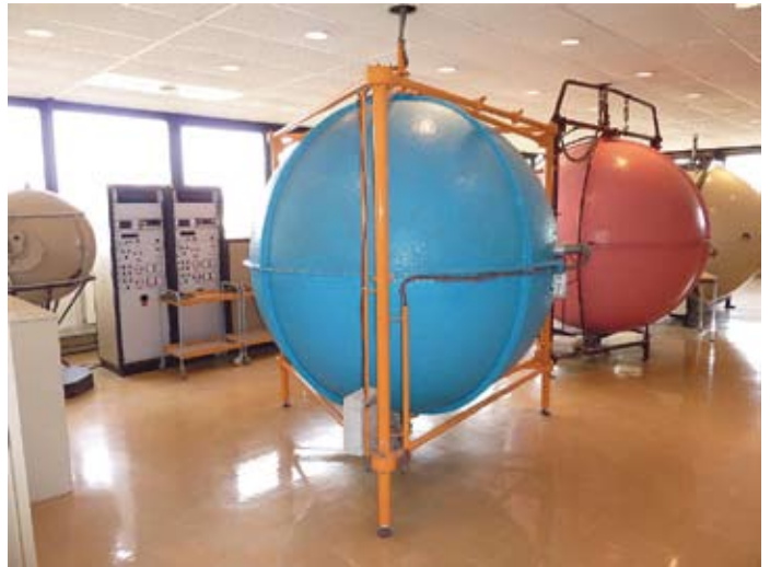
Measurement systems: Photometry department measures luminous flux and all other features of lamps as lamp current, color temperature etc.
